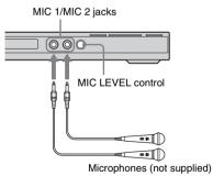
Before connecting a microphone, set the MIC LEVEL control to MIN (minimum).
